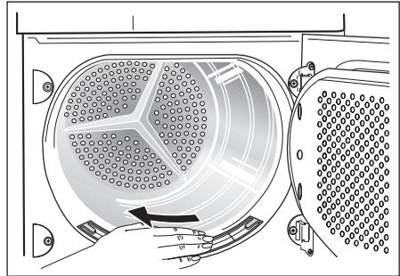
3. Remove the lint filter from the door by pulling the grip upwards.
